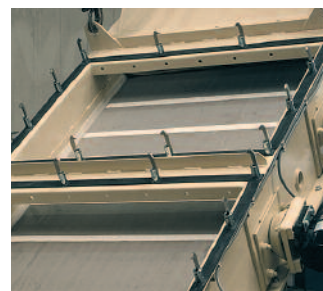
Screen mat with plastic protection within the area of the blow bars
